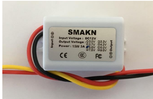
5VDC Voltage Regulator Required for reader power (see below) Pre-installed inside controller enclosure
